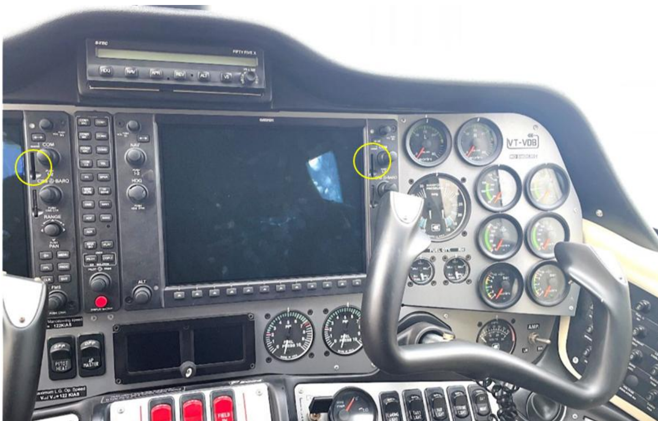
Fig 7: Aircraft’s cockpit photo post-accident (Two upper SD card slots without memory cards)
